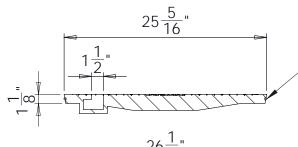
1/4" NEOPRENE O-RING GASKET GLUED INTO 1/4"x1/8" DEEP GROOVE MACHINED INTO COVER
